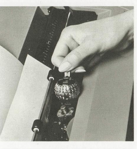
**Changing Typing Elements** Select the most appropriate style of type for each typing job. You can change the typing Element on your typewriter in seconds. Care should be taken not to drop the typing Element.
